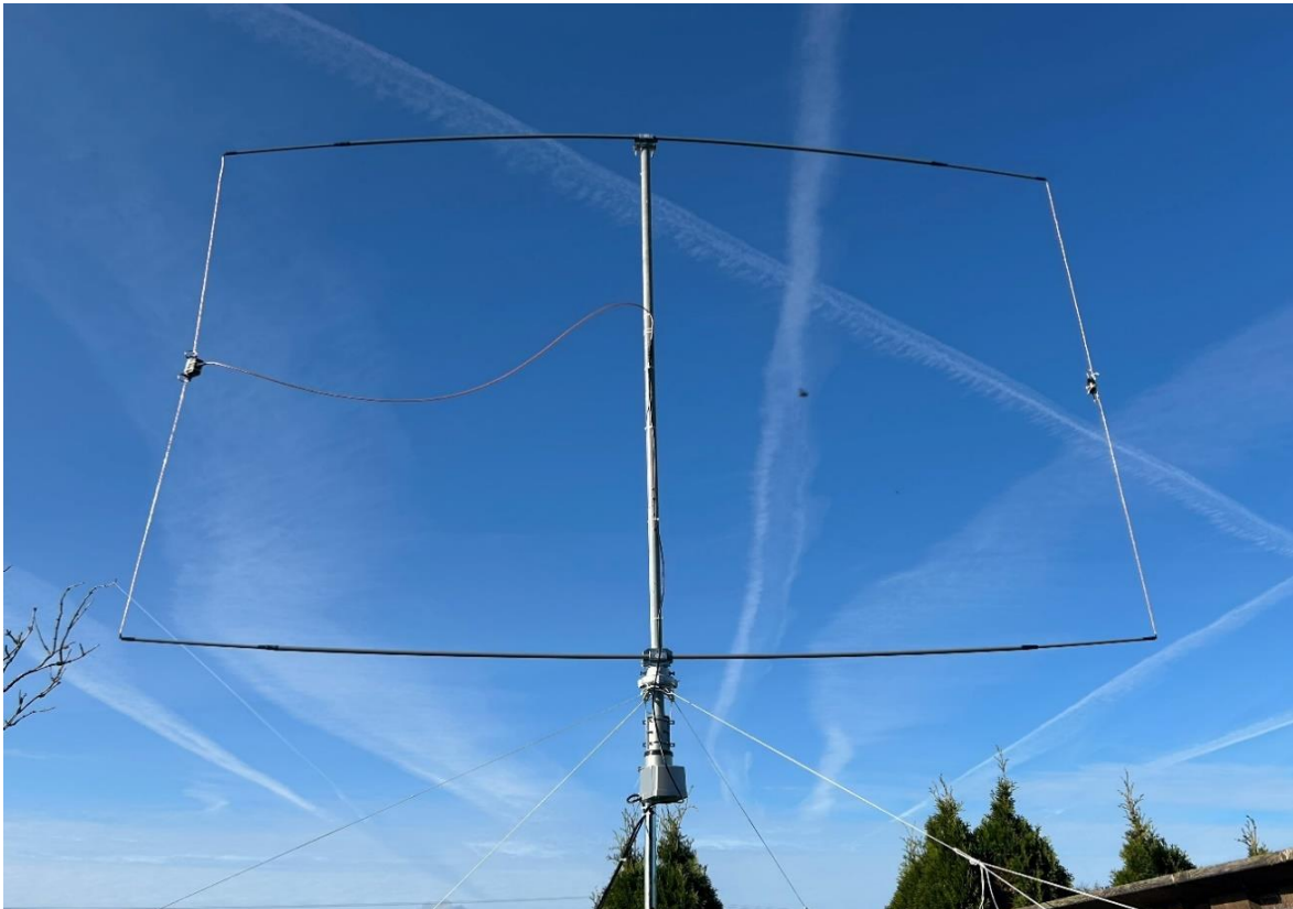
Fig.3: The "microFLAG" with rotator and thrust bearing on my small patio.
