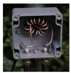
What will help is using a common mode choke at the bottom of the mast. Even better connect the shield of the coax to a ground stake at the bottom of the mast. That way the noise is guided to earth. You might add a common mode choke between that point and the coax going up the mast like this:
