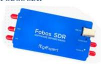
Hi, with some SDRs and with the SDR Server I provide non-native IQ rates. Actually very easy to take a native sample rate such as 4MHz and divide by 2, 4, 8 etc. (i.e. a power of 2). Other sample rates below 1 MHz are feasible by first diving 4 MHz by 4=1MHz, then using a fractional resampler. Assume you lose ~15% of bandwidth due to aliasing, 2 MHz = 1.7 MHz usable = Medium Wave spectrum.
