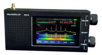
The USB port allows connection to a PC with CAT support, IQ data output and audio. You can use popular SDR softwares and transfet CAT and IQ data from SDR receiver to PC. There you can use more SDR SW features!
